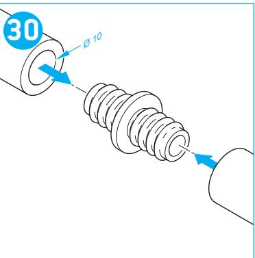
GB Connect the water tube to the water supply system with a hose bushing.
