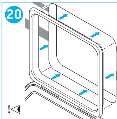
**GB** Check if the door frame fits • Remove the protective tape from the wall
