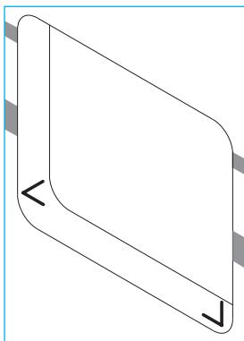
**GB** Saw cut-out. **NOTE 1:** Make sure this cut-out is perpendicular! **NOTE 2:** The cut-out panel from the wall is used as the door panel • Only saw in the indicated places!
