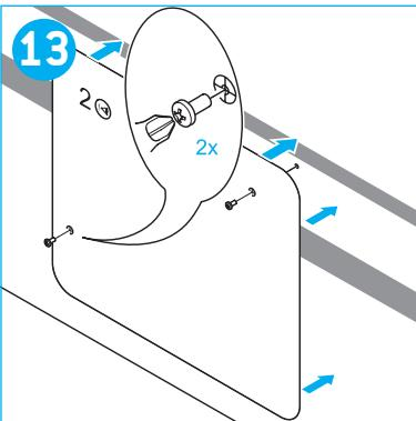
**GB Cut-out service door:** Place template 2 on the outside of the vehicle. Use the screw holes made in step 5 as reference.
