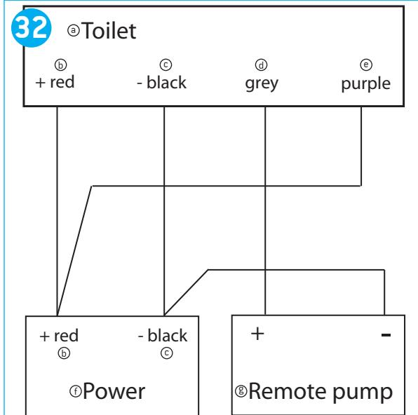
ⓘ Connect the wiring. If the toilet is connected to a pressurised system: Do not connect the grey and purple wire!
