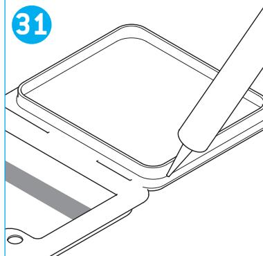
GB Fill the groove of the door outer with sealant.
