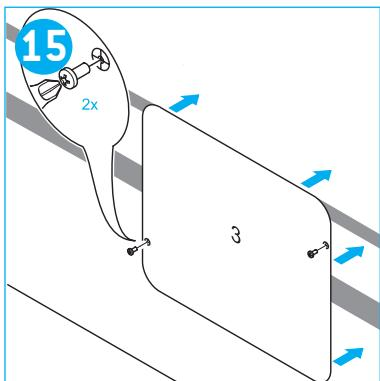
**GB** Place template 3 on the outside of the vehicle's wall. Use the screw holes made in step 5 as reference.
