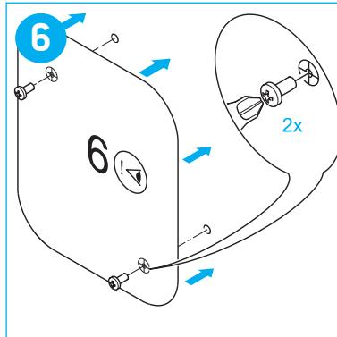
GB Cut-out water fill door: Place template 6 on the outside of the vehicle. Use the screw holes made in step 5 as a reference.
