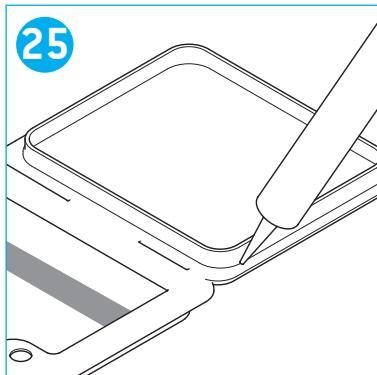
GB Fill the groove of the frame outer with sealant.
