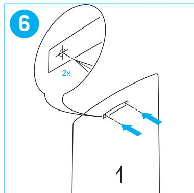
GB Mark the holes for the fastening strip • Remove template 1.
