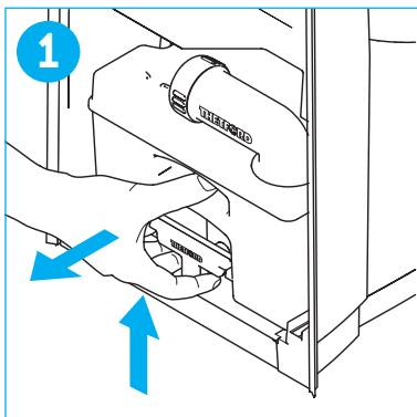
**GB** Remove the waste-holding tank • Take the plastic bag with four screws to connect the toilet out of the base • If applicable, remove the shower tray and adjust it in such a way that the C260 can be fitted onto it
