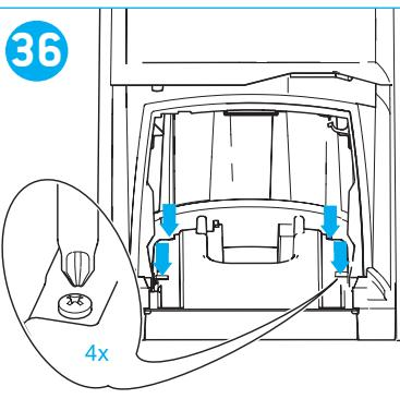
GB Screw the toilet to the floor, using 4 x 4,5 x 54mm.
