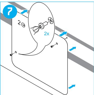
**GB** Cut-out service door: Place template 2 on the outside of the vehicle. Use the holes made in step 5 as a reference.
