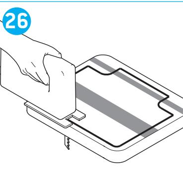
GB Saw the door panel • Remove the protective tape
