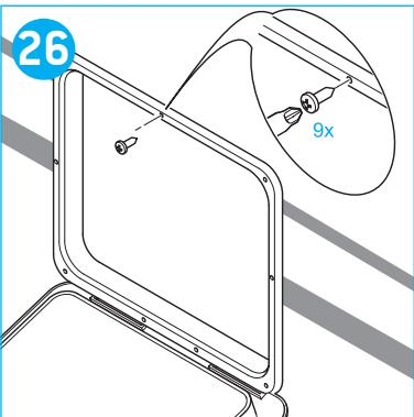
**GB** Screw the frame outer to the wall.
