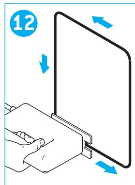
**GB** Saw the cut-out. **NOTE:** Make sure this cut-out is perpendicular!
