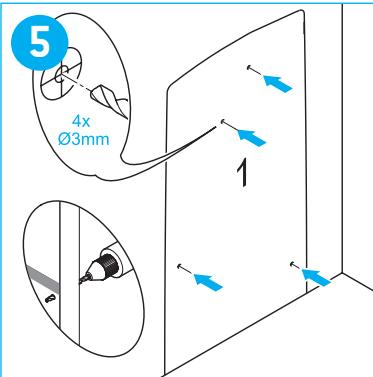
GB Drill four holes through the wall • Remove template 1
