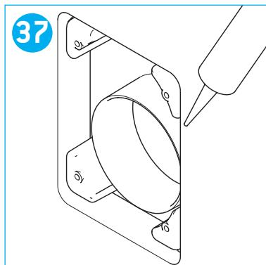
GB Place sealant around the cut-out of the water fill door.
