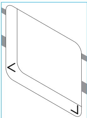
**GB** Saw the cut-out. **NOTE 1:** Make sure this cut-out is perpendicular! **NOTE 2:** The cut-out panel from the wall is used as the door panel. Only saw in the indicated places!
