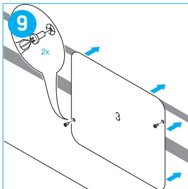
**GB** Place template 3 on the outside of the vehicle's wall. Use the holes made in step 5 as a reference.
