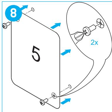
GB Place template 5 on the outside of the vehicle. Use the holes made in step 5 as reference.
