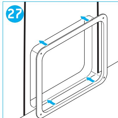
**GB** On the inside of the vehicle, connect the frame inner to the wall, either with screws or with double sided tape.
