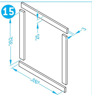
GB Aluminium strips are needed to strengthen the wall and to secure the door.
