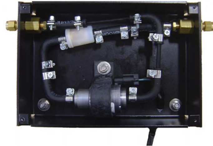
Fig. 20 Fuel Pump Enclosure Box
